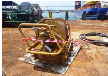
Damaged 10-Ton Winch after Base Plate Welds Failed Under Tension
